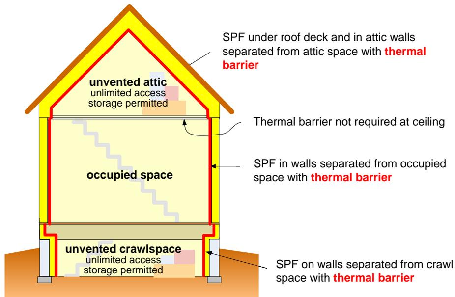
**FIGURE C2 – Thermal barrier requirements for unvented attics and crawlspaces with unlimited access or used for storage**
