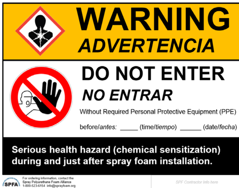
Figure 4: Example of Warning Sign
