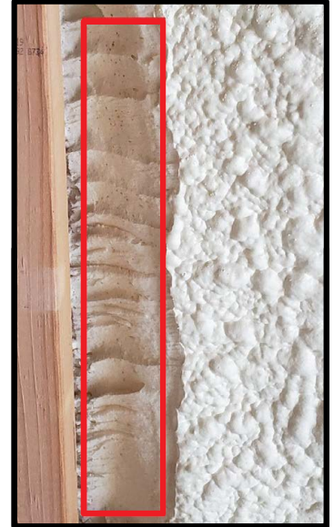
2.0 MAX sprayed at 4” The core of the foam will exhibit charring and enlarged cells with a fishy like odor.
