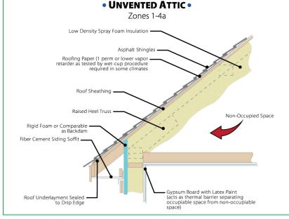
In unvented attic assemblies, the thermal envelope is continued from the lower-level walls up through the energy plates and risers (knee walls) onto the underside of the roof sheathing to fully encapsulate the attic space. The floor of the attic is left uninsulated. All soffit, ridge and gable vents are eliminated. The attic is now considered a component of the conditioned space. The drawing below illustrates an unvented attic assembly.
